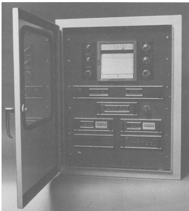
FIG. 13. Continuous yield measuring panel on centrifugal refining line.
